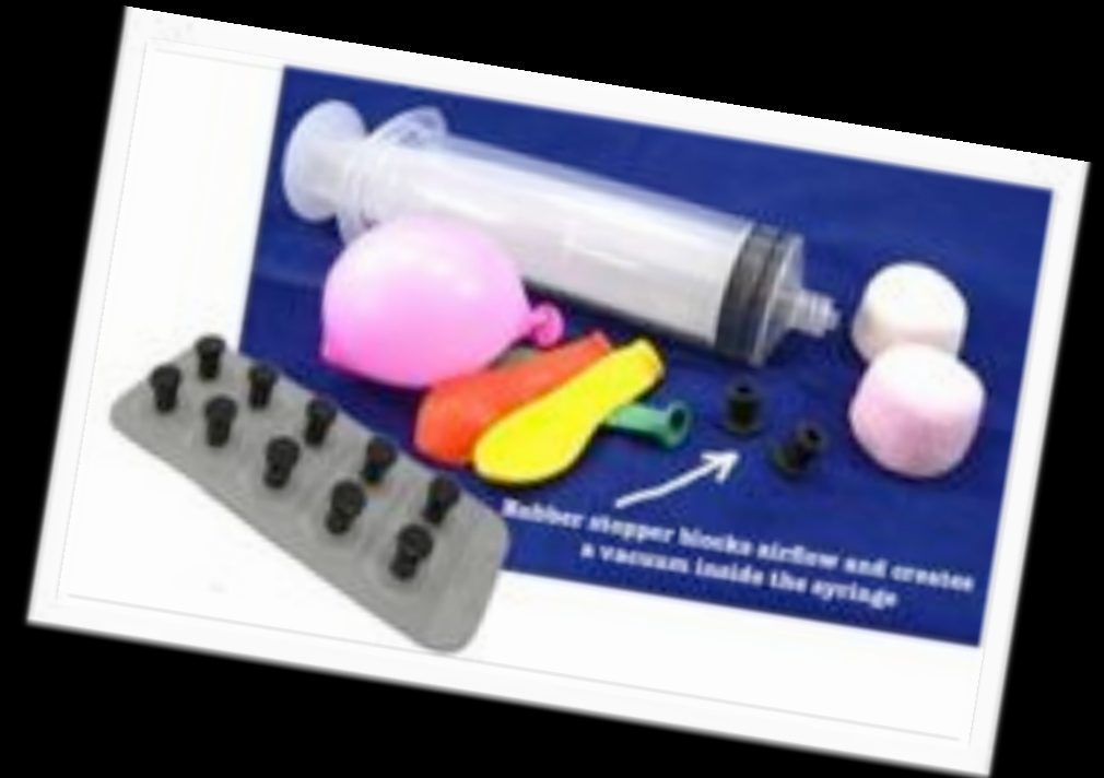
A syringe as vacuum chamber using vacuum stoppers
