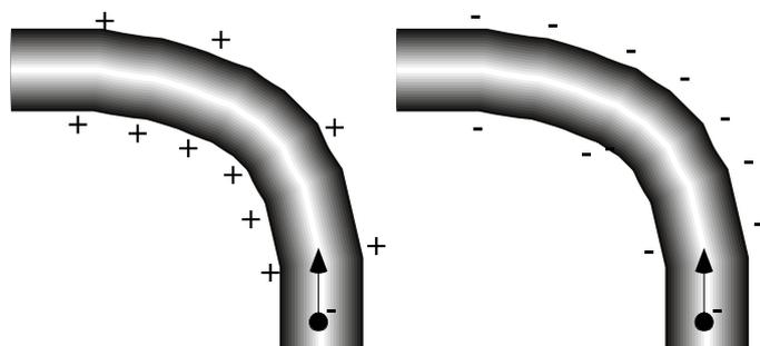
**Figure 4. Two ways to push a conduction electron around a corner**
