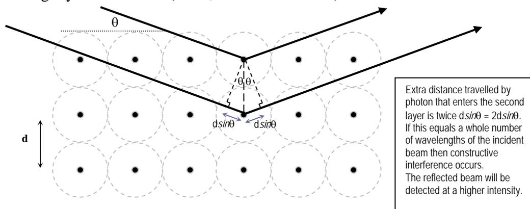
Although Bragg's law was used to explain the interference pattern of X-rays scattered by crystals, diffraction has been developed to study the structure of all kinds of matter with a beam, as long as the wavelength used is comparable to the spacing of the molecules (or atoms) within the object under investigation.
