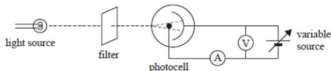
Emily uses various filters to shine a particular wavelength on the photocell. She increases the voltage (V) until the current just goes to zero and records this voltage. Emily repeats this process for different frequencies. Her results are shown in the table below.
