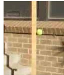
In an effort to reduce parallax the camera is usually set some distance from the object being filmed. When the lens is zoomed in, more light is required. Blurring can be the result making image identification difficult. The picture at right resulted from the camera zoomed in from some distance away. The tape measure is clear but the ball is blurred.
