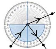
4. By gradually moving the light box from 0° around towards 90°, determine the incident angle at which the angle of refraction equals 90°. (In other words, find the **critical angle**.)
