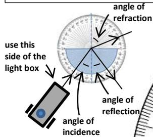
Note: The ray entering the perspex prism should not refract because it should enter at an angle of incidence of 0°.
