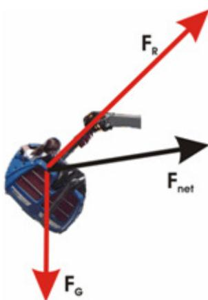
The diagram at right shows the situation near the *top* of the vertical motion. In this case the cart may even be above the horizontal, that is,  $\mathbf{F}_R$  has a downward component – at this point the cart is accelerating downward (whether still actually rising or falling) as well as inward.
