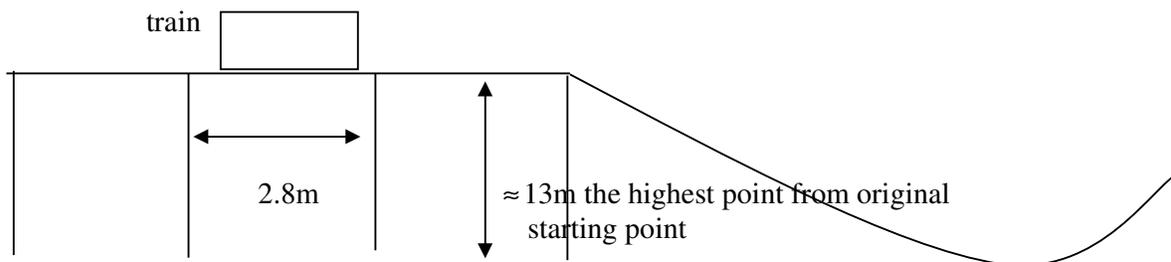
Time the train across at least 2 sections (one section being 2.8m) make sure this is measured using only the horizontal section of track.
