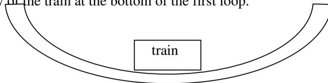
25. Assume the velocity of the train at this point is the same as the velocity at the bottom of the first hill (answer in question 15). Determine the reaction force by the track on the train at this point. (Net  $F = ma = mv^2/r$ )
