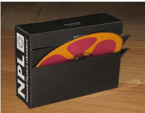
Slide a CD into the CD port, with the silver side towards the viewing window. Angle it so that the bottom edge is close to the viewing window.
