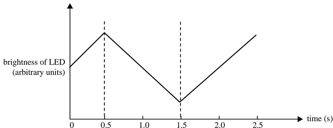
The important features that students were required to show were that the graph is inverted. That is, that increases in the resistance result in decreases in the brightness of the LED and since the stem stated that the diode is 'always conducting', the brightness should not go to zero at any point.
